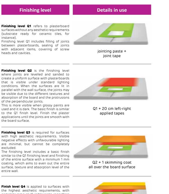
complete removal of visible joints, regardless of the type of lighting, and includes a base finish similar to finish level Q1 and covering the entire surface with a thin coat of up to 3 mm of moulding plaster.
