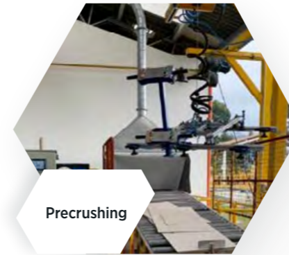
Hard waste grinding facility for flat sheets at the Etex Manizales plant (Colombia)
